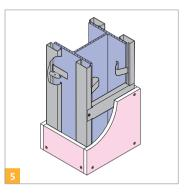
Cut short lengths of Gypframe GL1 Lining Channel (Figure 5), GFS1 Fixing Strap or Gypframe GFT1 Fixing 'T' (Figure 6) so as to form horizontal noggings to back board end joints.
