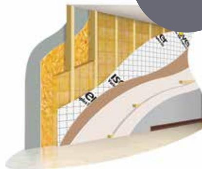
**Gyproc plasterboards are versatile when used as the internal lining to timber frame walls and allow for the creation of a void for the location of services.**
